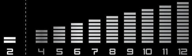
Adaptive protection level control sets the right protection level automatically in a range between 4 and 12. This is ensured by an additional brightness sensor which measures the intensity of the welding arc. This means that you are perfectly protected at all times, no matter what parameters you are welding with. Manual adjustments are no longer necessary.
